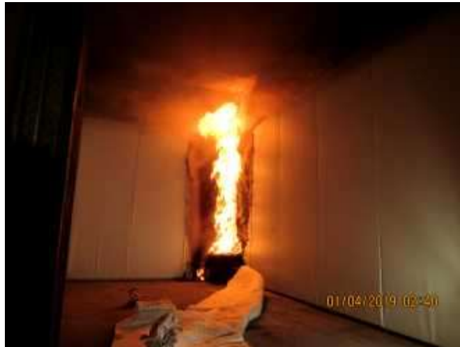
Photo No. 7 Increase in size of floor flame
