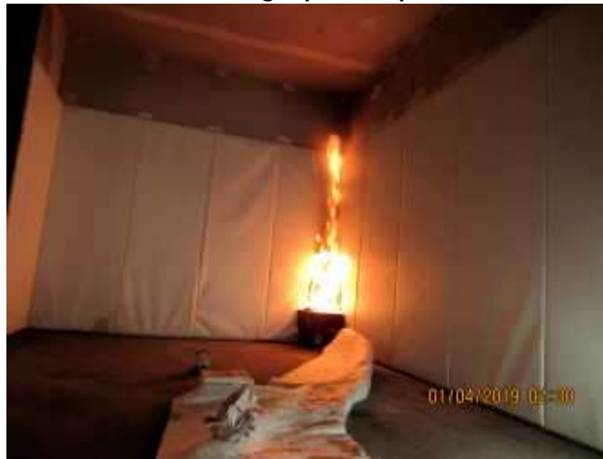
Photo No. 3 Flaming top of sample
